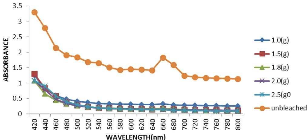
**Figure 4** Absorbance with varying weight of the mixture of Fuller’s earth and Activated carbon
