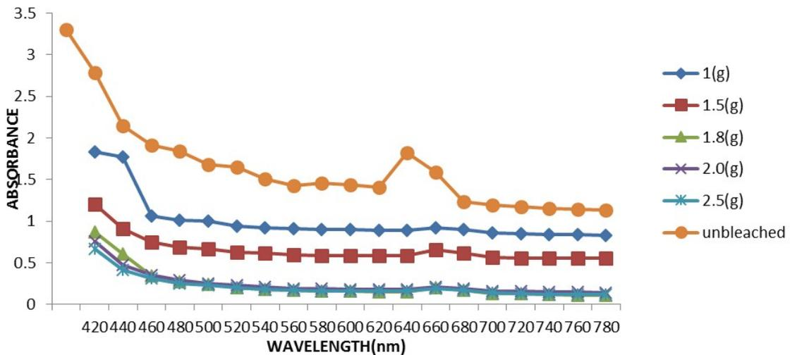
Figure 3 Absorbance with varying weight of Activated carbon
