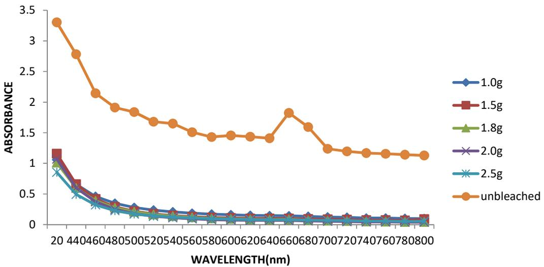
Figure 2 Absorbance with varying weight of Fuller's earth
