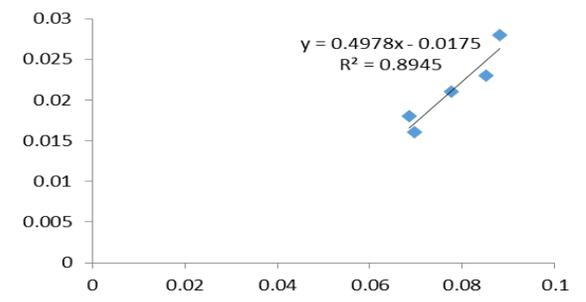
**Figure 8** Langmuir isotherm for bleaching with fuller's earth
